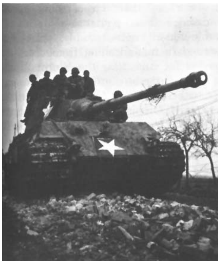
CAPTURED GERMAN TIGER (MARK VI) TANK with temporary U.S. markings. Note 88-mm. gun with flash hider.
