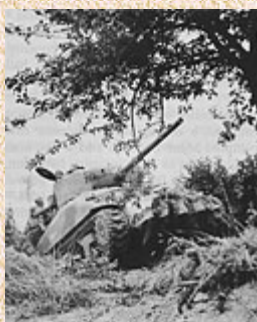
Rhino Tank with hedgerow cutter crashing through a hedgerow.
