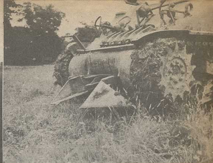
So the engineers got their heads together and came up with a plan. They told the Maintenance Battalion about it, and the maintenance men dreamed up a hedge-chopper for the Shermans.
