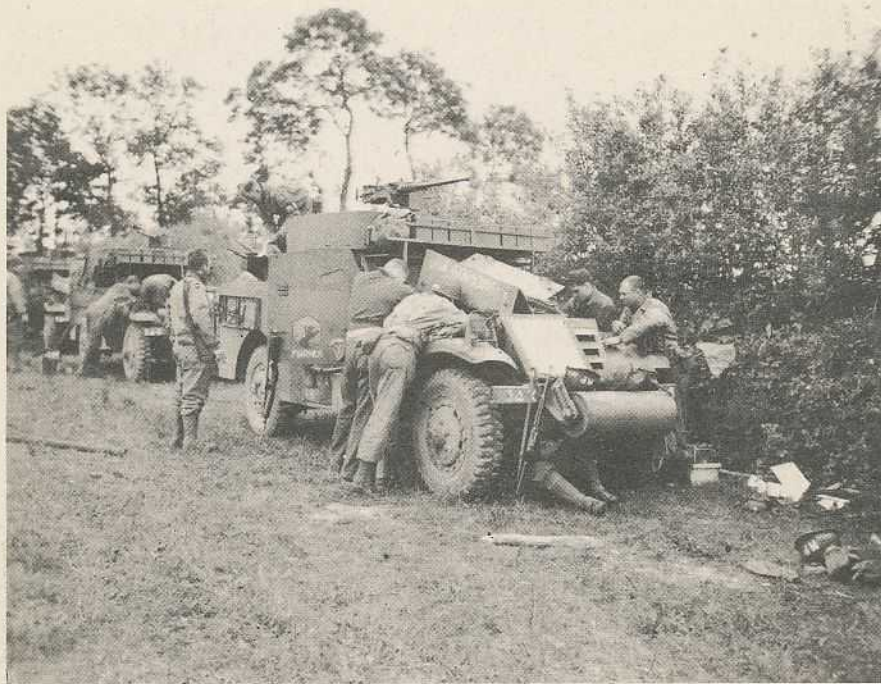
Within hearing of enemy artillery for the first time, division troops removed waterproofing on June 23-24.
